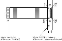
\* 37 pin D-SUB connector is the same as with the CN1.
