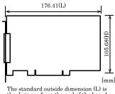
the distance from the end of the board to the outer surface of the slot cover.
