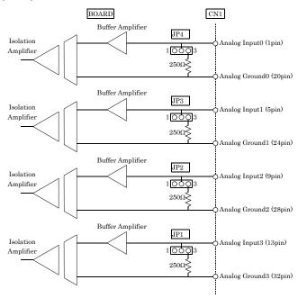
Analog signals are input to each channel via the isolation amplifier. This electrically isolates the channels from one another and this product's internal circuitry (PC) from the input pin.
