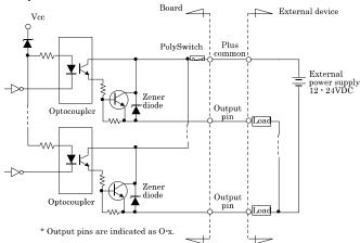
The output circuits of interface blocks of this product are illustrated in above Figure. The signal output section is an opto-coupler isolated open-collector output (current source type). Driving the output section requires an external power supply.
