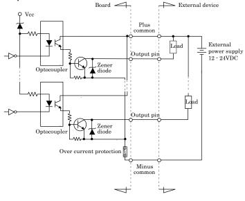
The output circuits of interface blocks of the PO-64L(PCI)H is illustrated in Figure. The signal output section is an opto-coupler isolated, open-collector output (current sink type). Driving the output section requires an external power supply.
