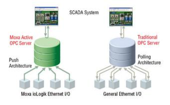
architecture, supports the standard OPC protocol, but also offers active (or "push") communication with Moxa's ioLogik series of Ethernet I/O products to HMI/SCADA systems, providing instant I/O status reports with "Active Tags." The event-driven active tags result in an I/O response time that is 7 times faster than other OPC Server packages, and results in an apparent 80% reduction in network traffic.
