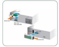
NE-4110: RJ45 Ethernet connector in stand-alone form factor
