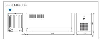
Bus Extender PCI bus Expansion Chassis (x4 Short size slots, On board Power)
