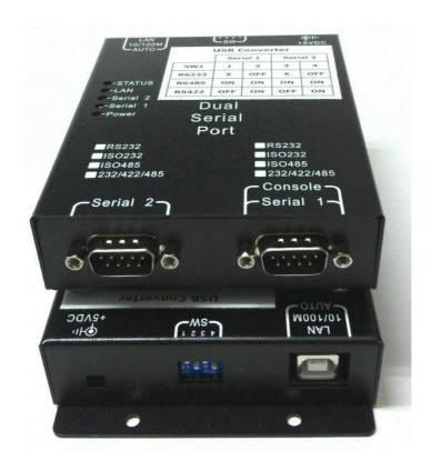
**★Support USB2.0** device controller **★512 Bytes FIFO** for data transfer **★Support data transmission LED display** for each port **★two Ground Isolated RS232** port for safety connection.
