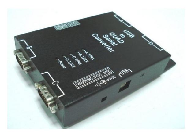
**★Support USB2.0** device controller **★512 Bytes FIFO** for data transfer **★Support LED display** for each port **★four RS232,RS422 and RS485** selectable port for remote connection.
