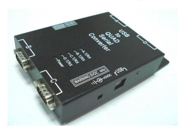
★Support USB2.0 device controller ★512 Bytes FIFO for data transfer ★Support LED display for each port ★four RS232 for local connection ★Support bus powered mode ★Use MOSCHIP MCS7840 chip
