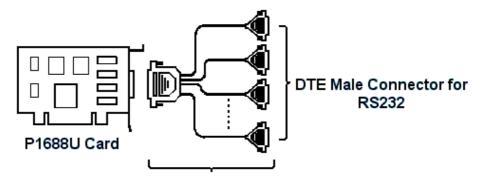
R801 Cable for 8 \* DB25 Male connector R804 Cable for 8 \* DB9 Male connector
