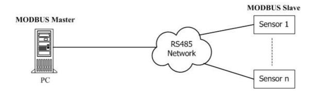
We have stored and forward interactive handshake feature in IS004S box. One master is serviced firstly and the other master will be serviced later. It is just like one MODBUS master to access and own one slave device independently.
