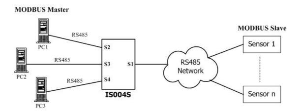
IS400S box will support RS232 interface. IS004S will support RS485 interface with GROUND isolated feature in all serial ports.
