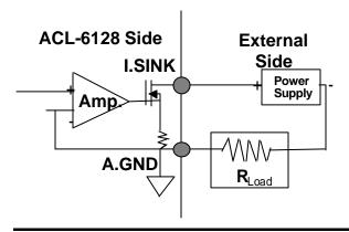
Note : For 4-20mA current sink mode, the output range should be set as Internal Reference with -5V and Unipolar mode.
