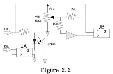
Each channel comes equipped with a pair of jumpers for either isolated or non-isolated selection. If the jumper plugs are installed on the upper posts of JAn, and JBn (n =0..15), the jumper n is configured as ISOLATED, otherwise the jumper plugs should be installed on the lower posts to configure as Non-isolated. Figure 3.4 are given here to illustrate how to configure the digital input channel 1 to 7.
