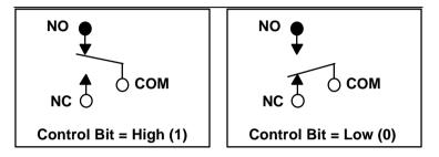
This relay has three contacts : NC (Normal Close), NO (Normal Open), and COM(Common). The CM post, located at the middle, can make contact either NO post or NC post. When the control bit is high (1), the COM post and NO post are contacted. If the control bit is low (0), the COM post and NC post make contact.
