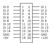
Figure 3.2 Pin Assignment of CN1
