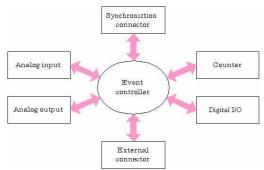
The arrows in the figure indicate the flow of control signals. The main control signals included clock signals and the operation start and stop signals.
