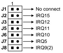
In factory jumper J1 is installed.
