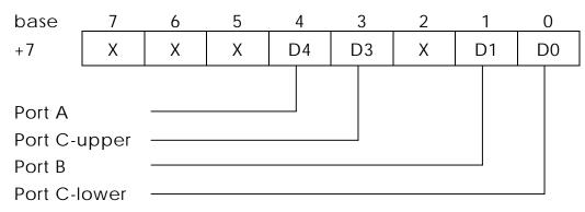
NotePA0 - PA7, PB0 - PB7 and PC0 - PC7 bits are<br/>associated to pins at J4 connector.X = don't care
