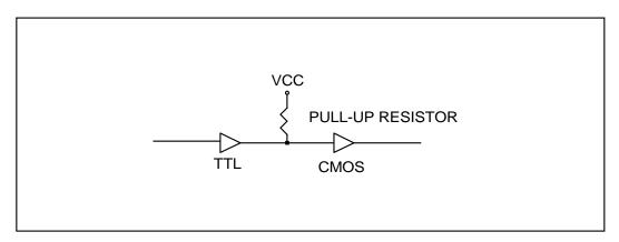
**Digital Input for Open/Short Switch Detection** – A pull-up resistor must be connected, especially at long distance wiring, to ensure logic high input level.
