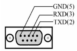
**Notice:** Due to the Hardware flow control problem will connecting some device just like PLC and it will caused TRP-C06 can't work, please take TRP-C06 's DB-9 PIN side (PIN 1,4,6 SHORT and 7,8 SHORT,
