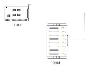
**Opt8J** is the RS-422/485 connection box with 8 port female DB25 connectors for MOXA 8 port boards, including the C168P. There are 8-DIP switches on the side of the Opt8J. Each switch controls the communication mode (RS-422 or RS-485) of each port, respectively.
