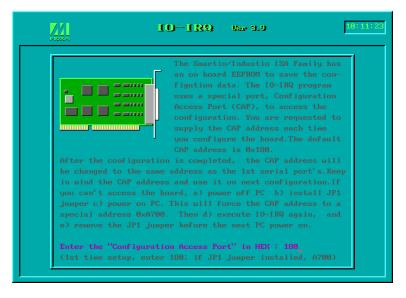
**3.** Enter the CAP address of the C168P board to be configured.
