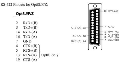
The RS-422 transmission distance can reach as long as 4000ft. The connection box needs an external power adapter to supply 5V DC power. Either 110V or 220V AC power adapter is selectable.
