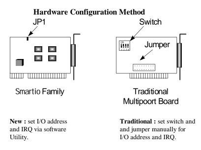
Instead of using traditional jumper or switch for IRQ and I/O address settings, hardware configuration of each port is easily set by DOS utility, **Io-irq.exe**, which reads and writes the on-board EEPROM for configuration information through the **CAP** (**Configuration Access Port**) address. The CAP address is the only channel via which the configuration utility Io-irq.exe can access the board, which is identical to **the first port's base I/O address**.
