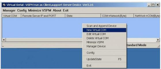
Step7. Select "Select Serial Port" and input TRP-C37M IP and port then press "OK".
