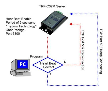
Step1: Run TRP-C37X DSM utility to set up the heart beat enable.
