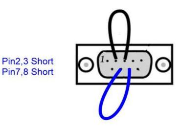
STEP1.RUN Virtual COM utility and set up the TRP-C37MA IP and PORT. STEP2.RUN TRPCOM test utility then select virtual-com port number. STEP3.Select terminal and key-in some word at "send command" text filed. STEP4.Click "Send Command" and get response.
