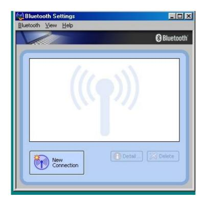
**Step5** Click on "New connection "icon into the Add New Connection Wizard, the USB dongle start to search all discoverable TRP-C51 units. Suppose just only 1 TRP-C51 unit need to be installed, we can see there is only one Bluetooth device been searched with the device name TRP-C51. Click "Next>" to continue.
