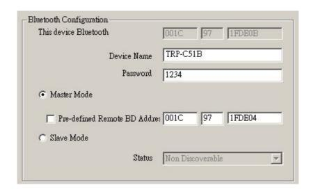
In TRP-C51 paired mode, it is necessary to set same name and password for both TRP-C51 (Master and Slave) .
