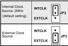
Figure 2.3 Timer's Clock Source Setting
