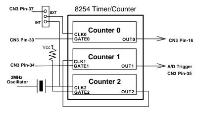
Figure 4.5 Block Diagram of 8254 Timer/Counter
