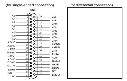
Figure 2.9.1 Pin Assignments of CN3
