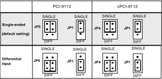
Figure 2.2 Analog Input Mode Setting
