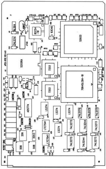
Figure 2.2 PCB Layout of the PCI-9112
