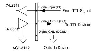
Figure 4.4 Digital I/O Connection
