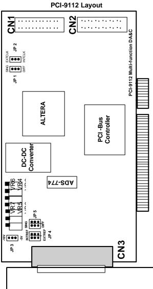
Figure 2.1 PCB Layout of the PCI-9112
