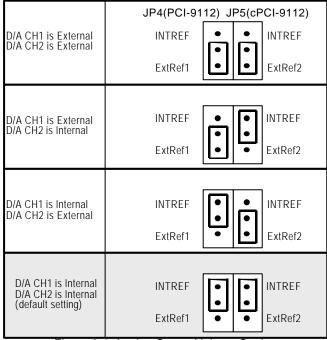
Figure 2.4 Analog Output Voltage Setting
