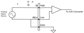
Figure 4.2.4 Floating source and differential input
