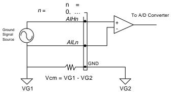
Figure 4.2.2 Ground source and differential input
