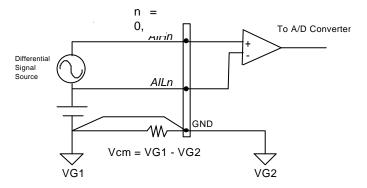
Figure 4.2.3 Differential source and differential input
