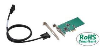
This product is a Low-Profile-size PCI bus expansion adapter (bundled with a 1m connection cable) that connects a PCI Express slot on a PC to a PCI bus expansion chassis.
