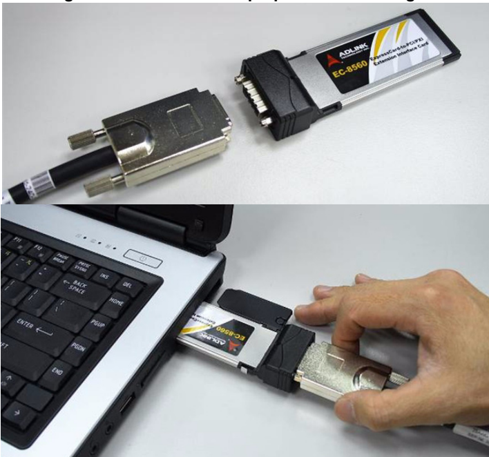
Figure 2-1: EC-8560 to Laptop Installation Diagram
