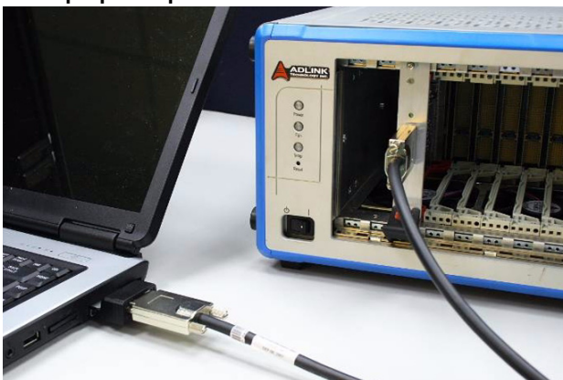
Figure 2-6: Laptop Computer Connected to a PXI™ Extension Chassis
