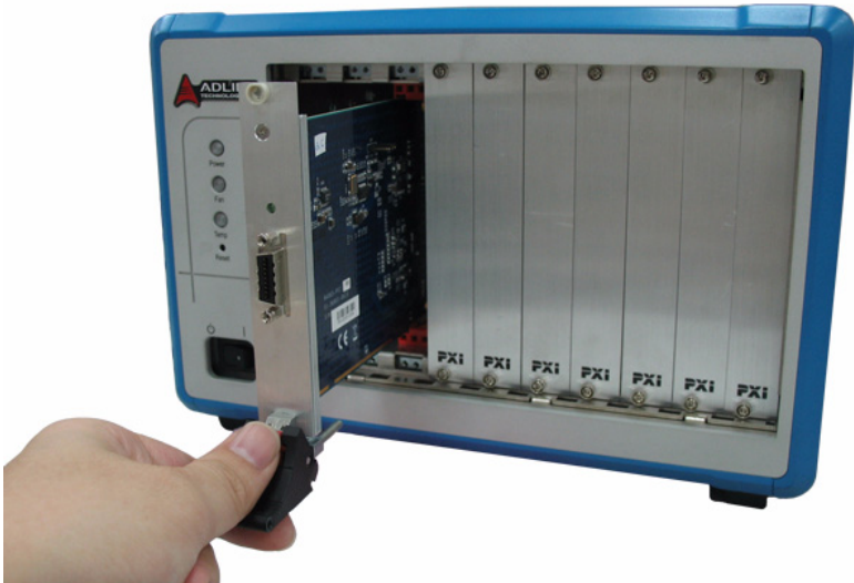
Figure 2-3: PXI-8565 to PXI Chassis Installation Diagram
