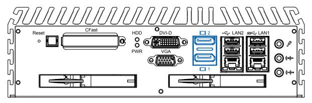
Each digital port is capable of driving resolutions up to 2560x1600 at 60 Hz through Display Port.
