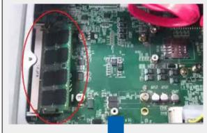
Tile the SODIMM module and insert it to the SODIMM socket.
