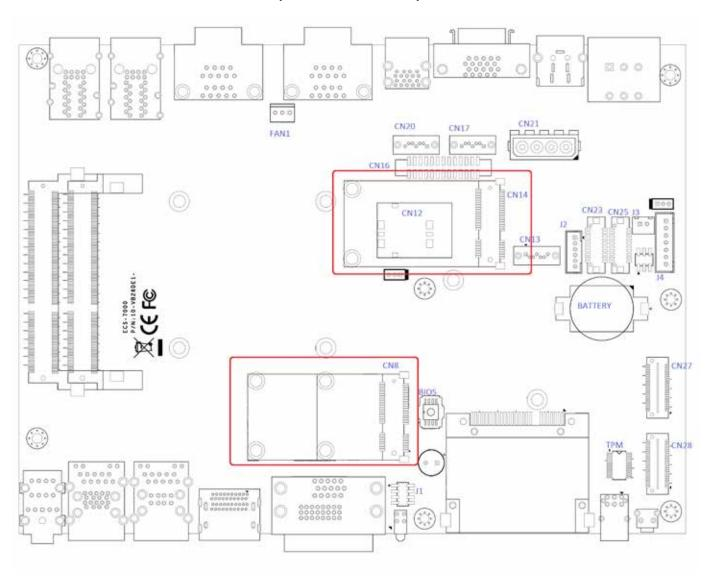
Both mSATA and Mini PCI-E share the same form-factor and similar electrical pinout assignments on their connectors. There was no clear mechanism to distinguish if a mSATA drive or a Mini PCI-E device is plugged into the socket until recently that SATA-IO issued an ECN change (ECN #045) to re-define pin 43 on mSATA connector as "no connect" instead of "return current path" (or GND).
