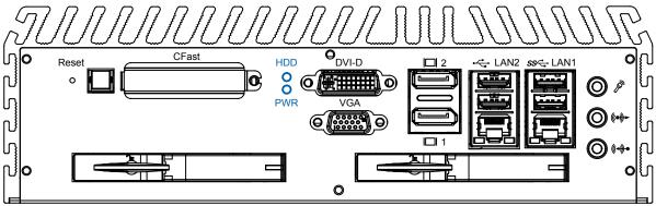
Yellow-HDD LED: A hard disk / CFast LED. If the LED is on, it indicates that the system's storage is functional. If it is off, it indicates that the system's storage is not functional. If it is flashing, it indicates data access activities.
