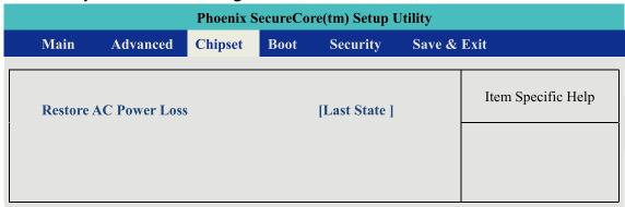
Figure 4.12: Power Loss Setu Screen
