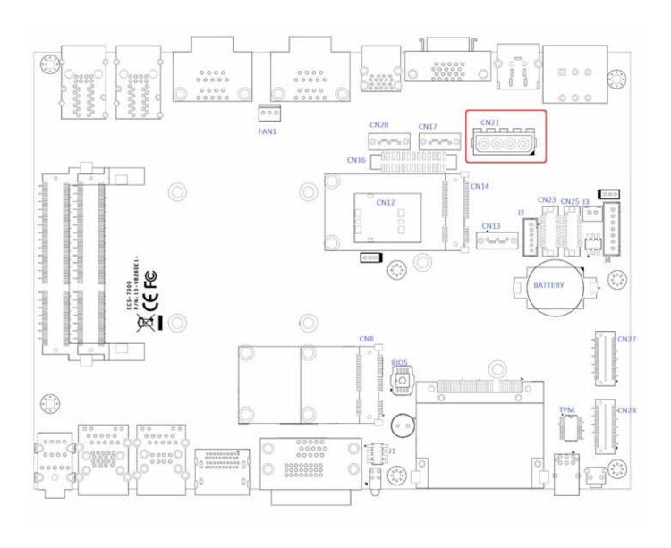
The ECS-7000 series is also equipped one SATA power connector. It supplies 5V (2A max.) and 12V (1A max) current to the hard drive or SSD.
