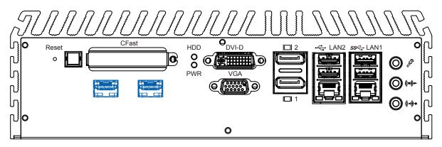
The SFP modules are input/output devices that plug into a Gigabit Ethernet (GE) port, linking the port with a 1000BASE-X fiber-optic network.
