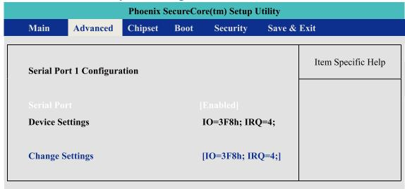
Figure 4.7: Serial Port 1Setup Screen
