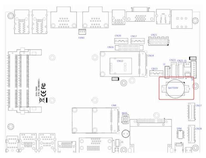
The ECS-7000 series' real-time clock is powered by a lithium battery. The battery is Panasonic BR2032 190mAh lithium battery. Replacing the lithium battery on your own is **NOT** recommended. If the battery needs to be changed, please contact with the Vecow RMA service team.
