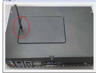
Put the ECS-7000 series upside down on a flat surface. You can see the "Pet-Door" exposed. Use a Philips screwdriver to loose the M3 flat-head screw on the "Pet-Door".
