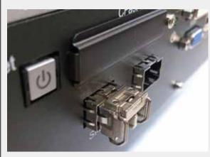
Pushing the Fiber module to the socket till it locked to the socket firmly. Repeat Step 2 if you are inserting a second SFP module. Do not remove the SFP module plugs until you are ready to install the cables.
