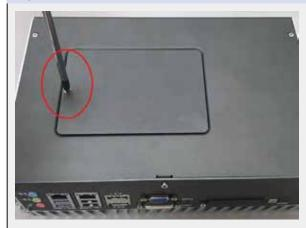
Tilt the HDD assembly and insert the wedge of HDD bracket to the bottom cover. Once it's firmly wedged, push it down and fix it using a M3 flat-head screw.
