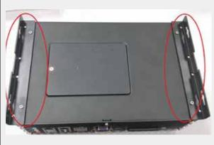
Fix two wall-mount brackets to the chassis with four M4 screws using a Philips screwdriver.
