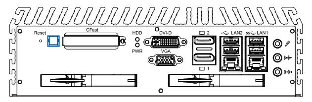
The power button is a non-latched switch with dual color LED (Blue/Orange) for indication S0, S3 and S5 status. Power button dual-color LED indicator:
