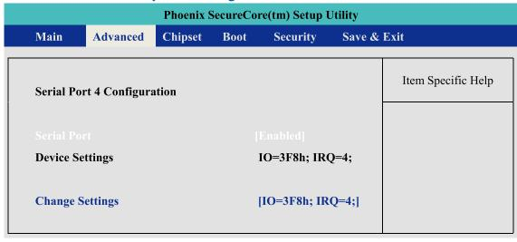
Figure 4.10: Serial Port 4 Setup Screen
