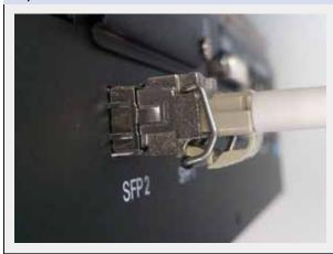
Loose the swing latch to unlock the Fiber Module and SC cable connection.
