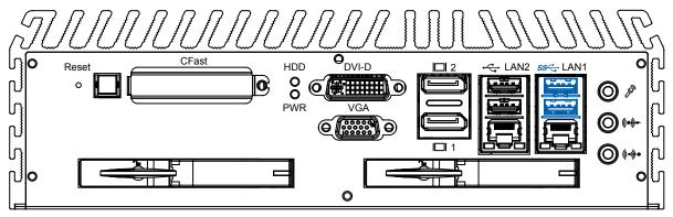
The ECS-7000 series comes with 2 USB 3.0 hosts on the front panel. These USB 3.0 ports allow data transfers up to 5 Gb/s. The controller supports SuperSpeed (SS), high-speed (HS), full-speed (FS) and los-speed (LS) traffic on the bus.
