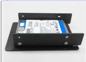
Place the HDD into the bracket and gently push it down to make it contact with thermal pad. Use a Philips screwdriver to fix the HDD with M3 screws. Please note that the HDD must be placed in the right direction as below.
