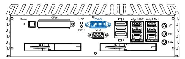
The DVI-D connector on the front panel supports both DVI and HDMI operation mode. This connector can either output DVI signals or HDMI signal. The DVI output mode supports up to 1920x1200 resolutions and HDMI output mode supports up to 1920x1200 resolutions. The DVI or HDMI mode is automatically selected according to the display device connected. You shall need a DVI-D to HDMI cable when connecting to a HDMI display device.
