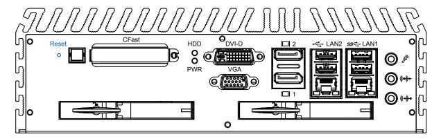
It is a hardware reset switch. Use this switch to reset the system without turning off the power. Momentarily pressing the switch will activate a reset.
