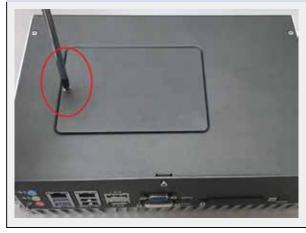
Put the ECS-7000 series upside down on a flat surface. You can see the "Pet-Door" exposed. Use a Philips screwdriver to loose the M3 flat-head screw on the "Pet-Door".
