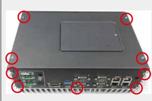
Use a screwdriver to loose 9 screws on the "Back Panel".
