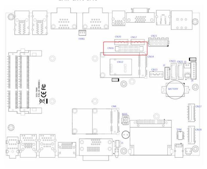
The ECS-7000 series offers 16 programmable I/O within TTL 5V tolerance. If the GPIO is logic high, it indicates that the mapping SIO GPIO pin is logic high level. If the GPIO is logic low, it indicates that the mapping SIO GPIO pin is logic low level.
