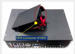
Pull out the SATA cable inside the chassis and connect it to HDD.
