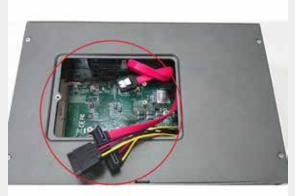
Remove the "Pet-Door" and you can see a SATA cable and DDR3 SODIMM socket exposed.
