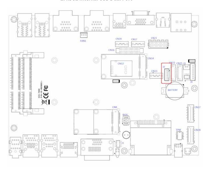
The ECS-7000 series' main board provides up to two USB plug-and-play ports for Dongle Key or LCD touch Panel using. The USB interface supports 480 Mbps transfer rate which complies with high speed USB specification Rev. 2.0, and fuse protection. The USB interface is accessed through one 1x6-pin JST 2.0mm connector. You will need an adapter cable if you use a standard USB connector. The adapter cable has a 1x6-pin connector on one end and a USB connector on the other.
