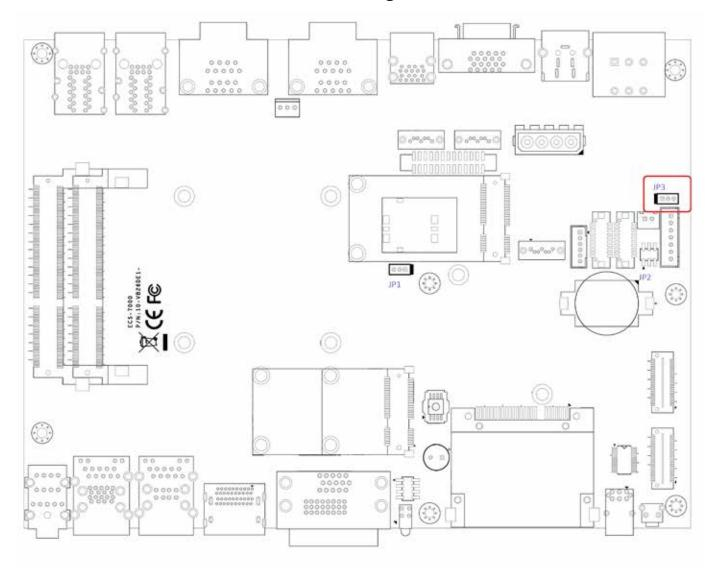
JP1 provides LVDS voltage selection function, closing Pin 1, 2 is for 3.3V LVDS power input; closing Pin 2, 3 is for 5V LVDS power input.
