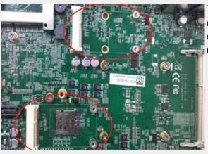
There are 2 Mini-PCIe sockets on the main board. Choose one of Mini-PCIe socket to put your mini-PCIe card in.
