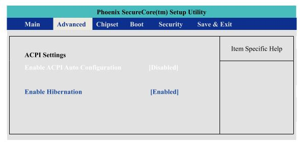
Figure 4.3: ACPI Setting Setup Screen
