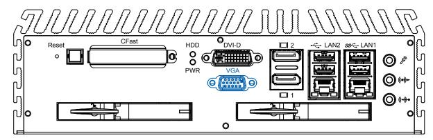
The ECS-7000 series comes with a DB15 female connector on the front panel to connect a VGA monitor. To ensure that the monitor image remains clear, be sure to tighten the monitor cable after connecting it to the ECS-7000 series . The VGA output mode supports up to 1920x1200 resolutions. The pin assignments of the VGA connector are shown below.
