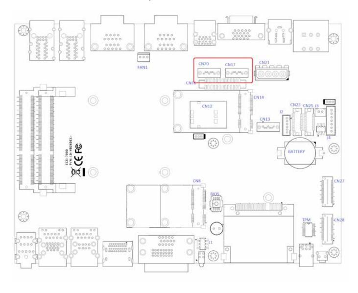
The ECS-7000 series features 2 high performance Serial ATA III interfaces that ease cabling to hard drives or SSD with thin and short cables while application need larger storage capacity.
