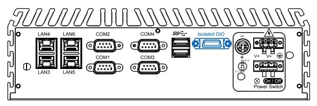
The ECS-7000 series offers an 16-bit DIO (8-DI / 8-DO) connector. Each bit of DI and DO equipped with a photocoupler for isolated protection. A power buffer device TPD2007F integrated in 8-DO circuit for motors, solenoids, and lamp drivers applications.
