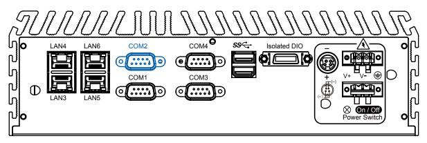
Serial port 2 can be configured for RS-232, RS-422, or RS-485 with auto flow control communication. Serial Port 2 default setting is RS-232, if you want to use RS-422 or RS-485, you can find the setting in BIOS.
