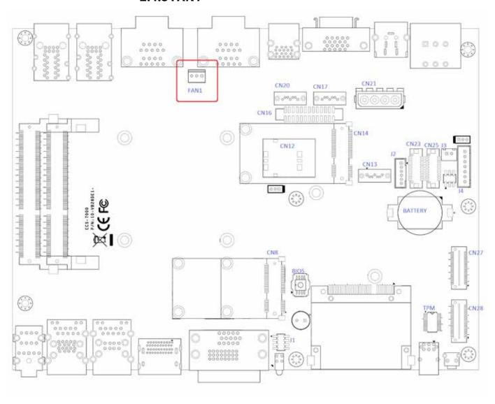
FAN power connector supports for higher thermal requirement.
