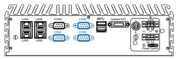
COM1, COM3 and COM4 are RS-232 only and provide up to 115200 bps baud rates. The pin assignments are shown in the following table:
