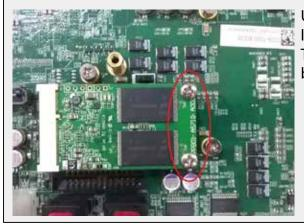
Using 2 BH-M2.5X6 screws to lock your mini-PCle card firmly. Then you can re-screw the back panel as the first step.
