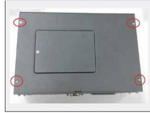
Put the ECS-7000 series upside down on a flat surface. Use a Philips screwdriver to loose screw on the back side.
