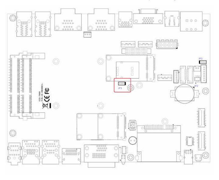
The ECS-7000 main board contains a jumper that can switch the AT/ATX Power Setting. Normally this jumper should be set with Pin 4 and Pin 6 in ATX power mode. And power on the system by the 2-pin terminal block at the top panel. If you set it with Pin 2 and Pin 4 in AT power mode. It will send the power button signal to power on the system automatically
