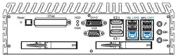
The 10/100/1000 Mbps Ethernet LAN ports 1 and 2 use 8-pin RJ-45 connector. LAN1 is equipped with Intel 82579LM for AMT function. LAN2 is equipped with Intel 82574L. Using suitable RJ-45 cable, you can connect ECS-7000 sereis system to a computer, or to any other piece of equipment that has an Ethernet connection, for example, a hub or a switch. Moreover, both of them have Wake-on-LAN and Preboot Execution Environment capabilities. The following diagram shows the pinouts for LAN1 and LAN2 port.
