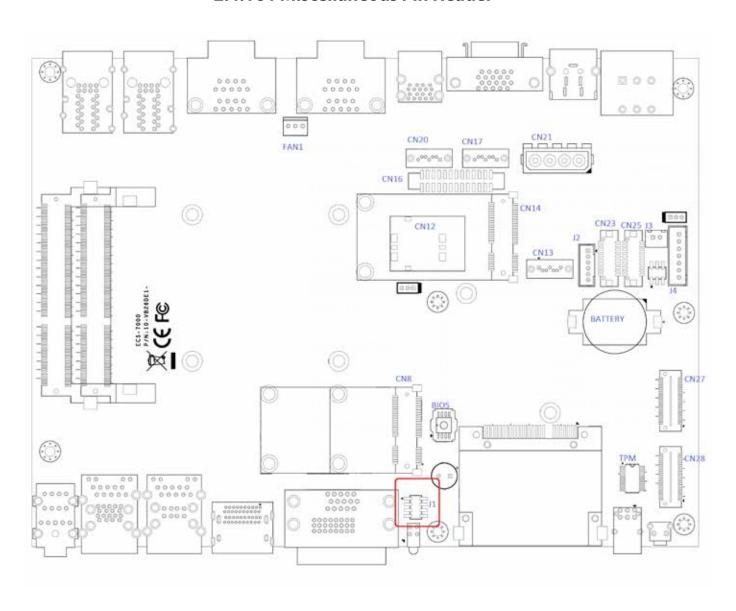
These pin headers can be used as a backup for the following functions: hard drive LED indicator, reset button, power LED indicator, and power-on/off button. The front and top panel already provides access to these functions. The following table shows the pinouts for Miscellaneous port:
