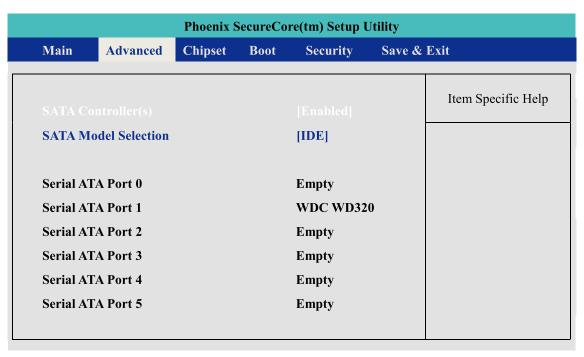
Figure 4.6: SATA Configuration Setup Screen
