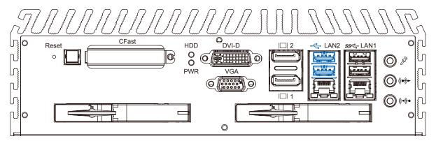
The ECS-7000 series comes with 2 USB 2.0 hosts on the front panel. The USB interface supports Plug and Play, which enables you to connect or disconnect a device whenever you want, without turning off the system. The hosts can be used for an external flash disk or hard drive for storing large amounts of data. You can also use these USB hosts to connect to a keyboard or a mouse. The following diagram shows the pinouts for USB1 and USB2 port.
