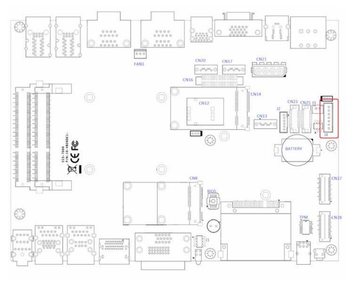
The LCD inverter is connected to J4 via a JST 7-pin, 2.5mm connector to provide +5V/+12V power to the LCD display.
