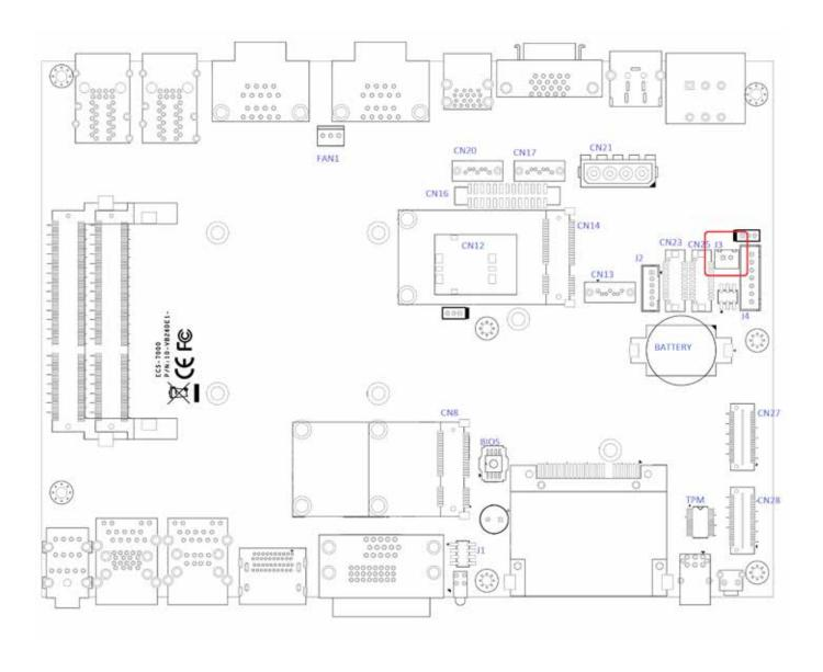
The ECS-7000 series is also equipped one SATA DOM power connector. It supplies 5V (0.5A max.) current to the SATA DOM.
