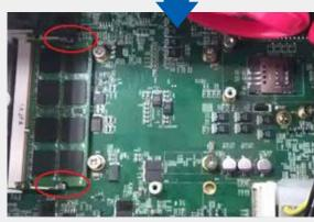
As it's firmly contacted with socket connectors, press it down until the clamps of the socket snap into the latching position of SODIMM module.
