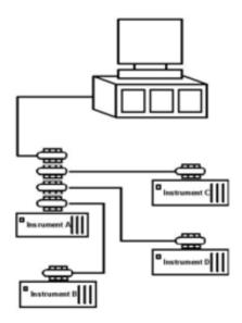
Figure 2-6: LPCIe/LPCI-3488A Star Connection Configuration
