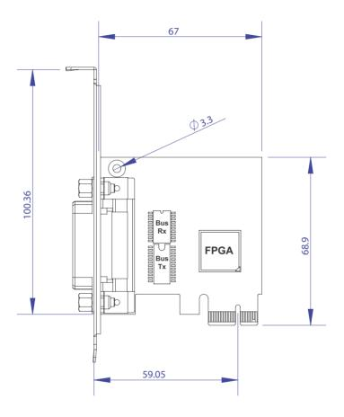
Figure 2-2: PCB Layout of the LPCle-3488A
