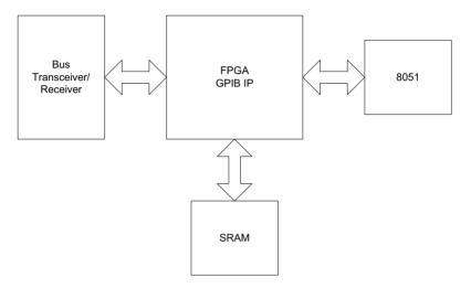
Figure 3-4: USB-3488A Block Diagram
