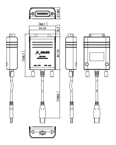
Figure 2-3: Layout of the USB-3488A
