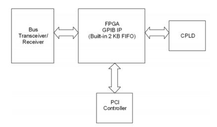
Figure 3-3: LPCI-3488A Block Diagram
