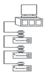
Figure 2-4: LPCIe/LPCI-3488A Linear Connection Configuration
