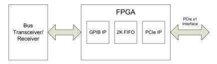
Figure 3-2: LPCle-3488A Block Diagram
