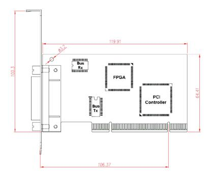
Figure 2-1: PCB Layout of the LPCI-3488A
