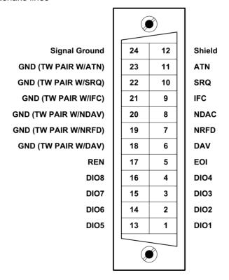
Figure 3-1: Standard GPIB Connector
