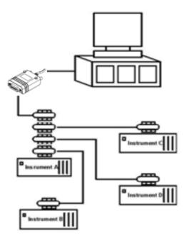
Figure 2-7: USB-3488A Star Connection Configuration
