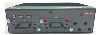
2. Align the CFast card with the socket guide.
