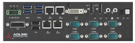
Figure 1-6: Front Panel I/O
