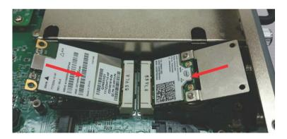
5. Seat the mini-PCI-E wireless module and use the 4 included M2.5-P-head-L5 screws to fix.
