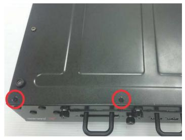
2. Remove the 4 fastening screws from the top cover edges.
