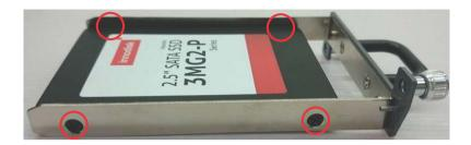
5. Re-insert the rack and gently slide inward until the SATA connector is engaged.
