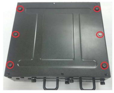
2. Use the 6 provided M4 screws to fix the 2 wall-mount brackets to the chassis according to the spacing of the screw holes and brackets, as shown.
