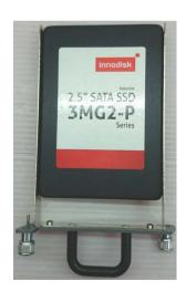
4. Fix the HDD or SSD to the rack using the 4 included M3 screws.
