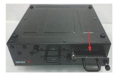
3. Seat the HDD or SSD in the HDD rack.
