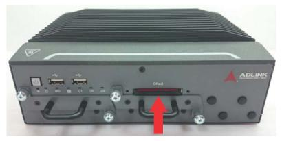
4. Replace the cover and the 2 fastening screws.
