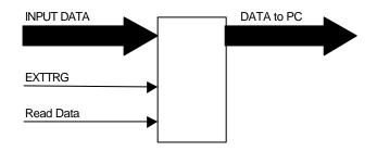
Figure 4.1 External Trigger Function Block
