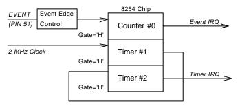
Figure 4.3 Timer / counter system of PCI-7396.
