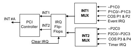
Figure 4.4 Dual Interrupt System of PCI-7396
