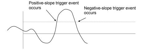
Figure 4.8 Analog trigger conditions
