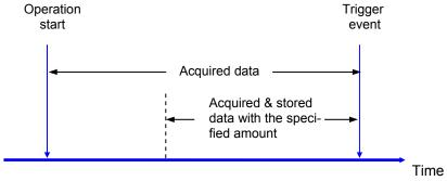
Figure 4.2 Pre trigger (the trigger event occurs after the specified amount of data has been acquired)
