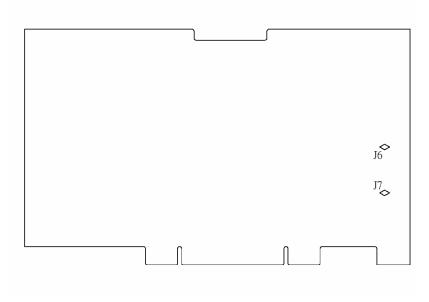
Figure 3.2: Location of solder switches
