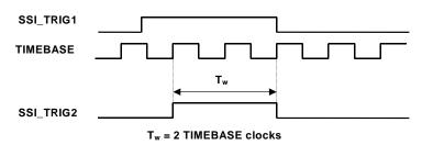
Figure 4.14 SSI TRIG2 output signal timing
