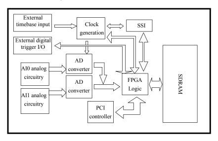
Figure 1.1: PCI-9820 block diagram
