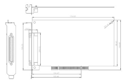
Figure 1-1: PCI-6208V-GL/6216V-GL Rev. C2 Layout
