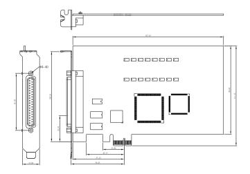
Figure 1-2: PCle-6208V/6216V-GL Layout
