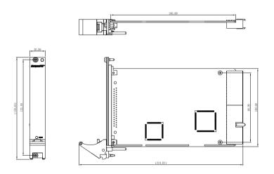
Figure 1-4: cPCI-6208V/R-GL and cPCI-6216V/R-GL Layout
