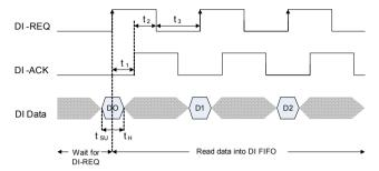
$t_{\,\text{SU}}\,$  = Maximum required setup time
