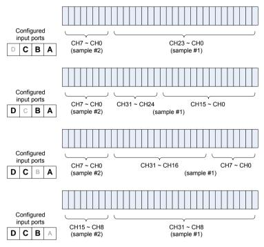
Figure 3-4: DI Row Data Mapping for 24 bits Data Width
