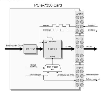
Figure 3-16: DO Handshaking Mode Architecture
