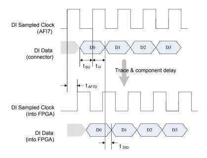
$t_{\text{AF7D}}$  = Time delay of external sampled clock from AFI7 to internal
