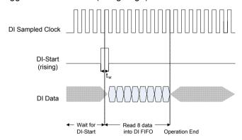
tw = Minimum required pulse width time
