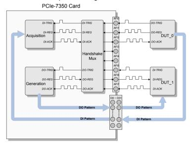
Figure 3-37: Configured AFI as Handshaking Interface
