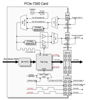
Figure 3-20: DO Burst Handshaking Mode Architecture
