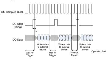
tw = Minimum required pulse width time
