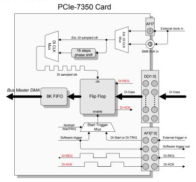
Figure 3-18: DI Burst Handshaking Mode Architecture
