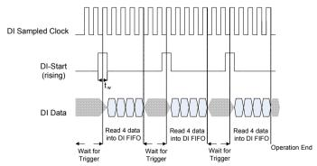
$t_w$  = Minimum required pulse width time
