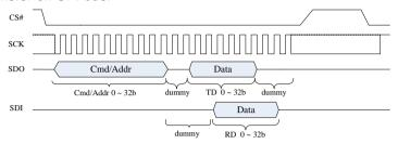
Figure 3-32: Data Transfer on SPI Bus
