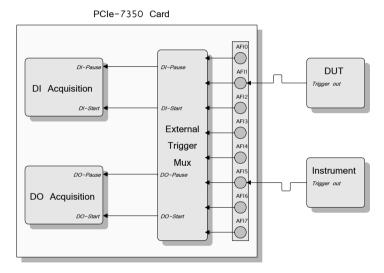
Figure 3-34: External Digital Trigger Input Configuration
