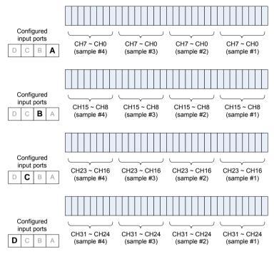
Figure 3-2: DI Row Data Mapping for 8 Bits Data Width
