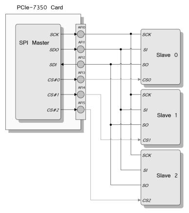
Figure 3-31: SPI Master of PCIe-7350
