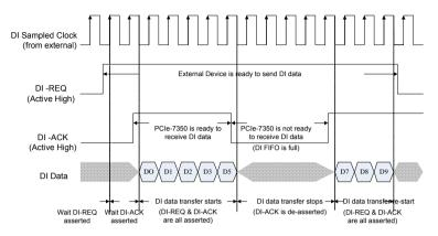
Figure 3-19: DI Burst Handshaking Timing Diagram
