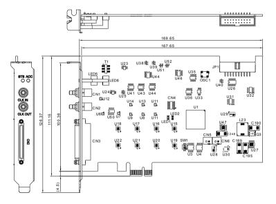
Figure 2-1: PCB Layout and Mechanical Drawing of the PCle-7350
