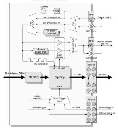
Figure 3-12: DO Continuous Mode Architecture
