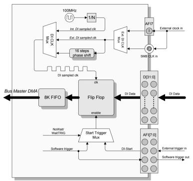
Figure 3-10: DI Continuous Mode Architecture
