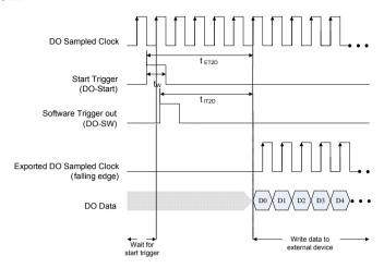
tw = Minimum detectable trigger width
