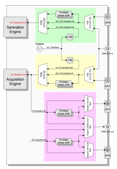
Figure 3-9: DI/DO Sample Clock Architecture
