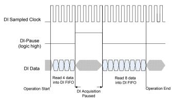
Figure 3-26: DI Gated Trigger
