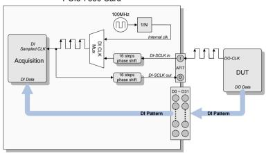
Figure 3-38: Configured AFI7 as DI Sampled Clock In/Out
