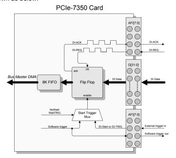
Figure 3-14: DI Handshaking Mode Architecture
