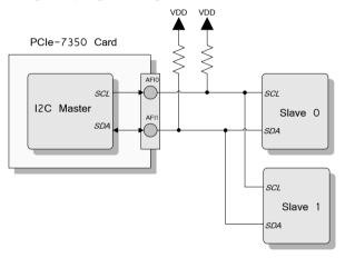
Figure 3-28: I2C Master of PCIe-7350
