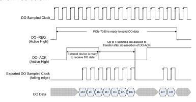
Figure 3-21: DO Burst Handshaking Timing Diagram
