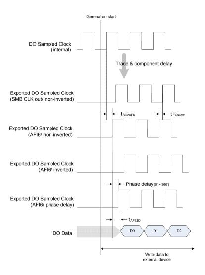
t<sub>SC2AF6</sub> = Time delay from sampled clock (internal) to exported sampled clock (AFI6)
