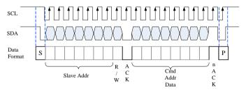
Figure 3-29: Data Transfer on the I<sup>2</sup>C Bus
