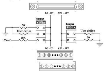
Figure A-2: Resistor Termination Schematic
