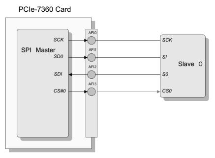
Figure 3-32: SPI Master of PCIe-7360
