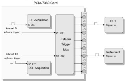
Figure 3-36: Configured AFI as Internal Software Trigger Output
