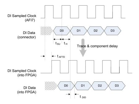
$t_{AF7D}$  = Time delay of external sampled clock from AFI7 to internal  $t_{DID}$  = Time delay of DI data from VHDCI connector to internal
