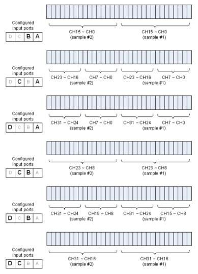
Figure 3-3: DI raw data Mapping for 16-Bit Data Width
