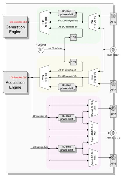
Figure 3-9: DI/DO Sample Clock Architecture
