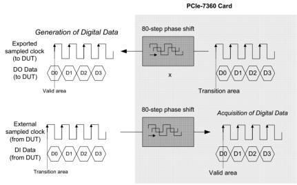
Figure 3-6: Phase Shift of Sample Clock
