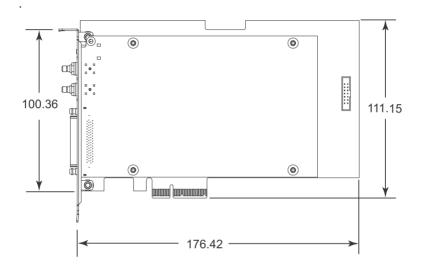
Figure 1-3: PCIe-7360 Schematic Diagram
