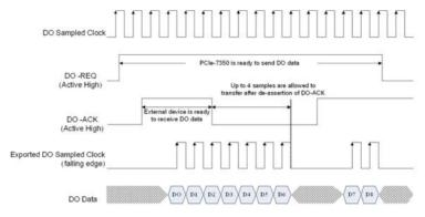
Timing of DO DMA in burst handshake mode is as shown.
