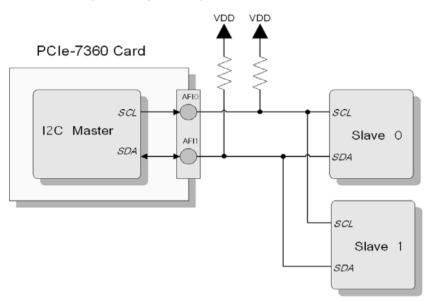
Figure 3-29: I2C Master of PCIe-7360
