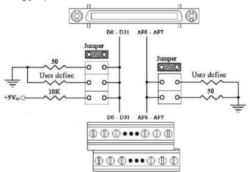
Figure A-2: Resistor Termination Schematic
