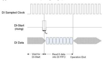
tw = Minimum required pulse width time
