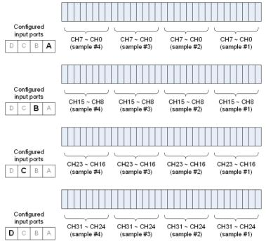
Figure 3-2: DI Raw Data Mapping for 8-Bit Data Width
