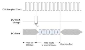
tw = Minimum required pulse width time
