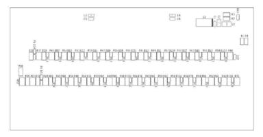
Figure A-3: DIN-68H Layout (Back Side)
