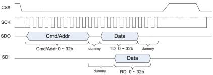
Figure 3-33: Data Transfer on SPI Bus
