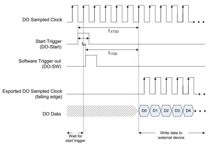
tw = Minimum detectable trigger width
