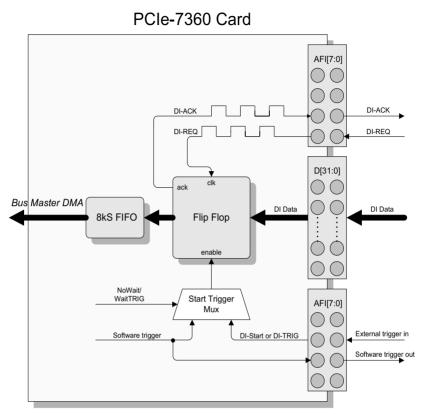
Figure 3-14: DI Handshake Mode Architecture
