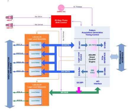
Figure 3-1: PCIe-7360 Block Diagram
