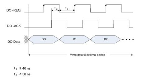
Timing of DO DMA in handshake mode is as shown.
