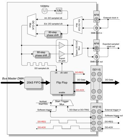
Figure 3-20: DO Burst Handshake Mode Architecture
