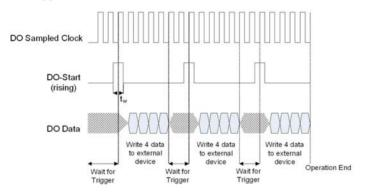
$t_w$  = Minimum required pulse width time
