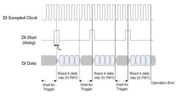
tw = Minimum required pulse width time
