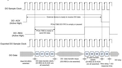
Figure 3-22: DO Burst Handshake 2 Timing Diagram
