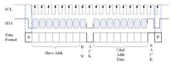
Figure 3-30: Data Transfer on the I<sup>2</sup>C Bus
