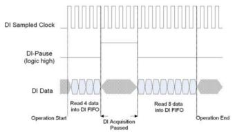
Figure 3-27: DI Gated Trigger
