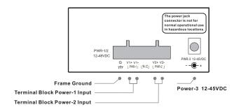
\*Note<sup>1</sup>: The power jack connector is not for normal operational use in hazardous locations.
