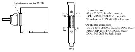
Connecting an Interface Connector and Connectors That Can Be Used
