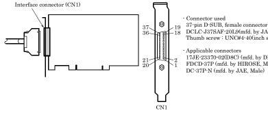
DCLC-J37SAF-20L9(mfd. by JAE) Thumb screw : UNC#4-40(inch screw) Applicable connectors 17JE-23370-02(D8C) (mfd. by DDK, Male) FDCD-37P (mfd. by HIROSE, Male) DC-37P-N (mfd. by JAE, Male)
