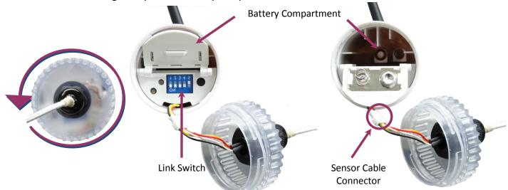
**Note:** When separating the base, be careful to ensure the sensor cable connector stays connected.
