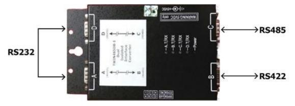
1) When one RS422 device need to work in RS485 network, we can use TWIN485DB-I box as such converter box. One set of module in TWIN485DB-I box is set in RS232 to RS422 interface converter function. The other set of module in TWIN485DB-I box is set in RS232 to RS485 interface converter function. Then we can use one NULL MODEM cable between two RS232 ports. So we can have RS422 to RS485 interface converter available.
