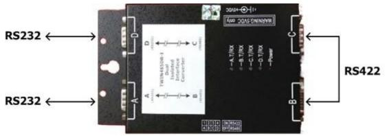
When we need to connect two RS232 device with GROUND isolated feature, we can set TWIN485DB-I box as two sets RS232 to RS422 interface converter. Then we can use one NULL MODEM cable between two RS422 ports. So two RS232 ports will be used as RS232 isolator.
