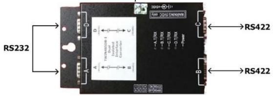
When we need to extend the range for RS422 connection, we can set TWIN485DB-I box as two sets RS232 to RS422 interface converter. Then we can use one NULL MODEM cable between two RS232 ports. So two RS422 ports will be used as RS422 repeater.
