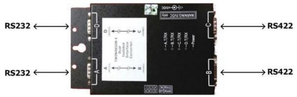
Now you can have two RS232 devices to connect with remote device via RS422 interface connection.
