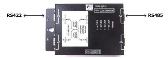
We can use port D as RS422 input (DIP Switch bit4 set in ON location) and port C as RS485 output (DIP Switch bit3 set in OFF location) to let one RS422 device to work in RS485 network.
