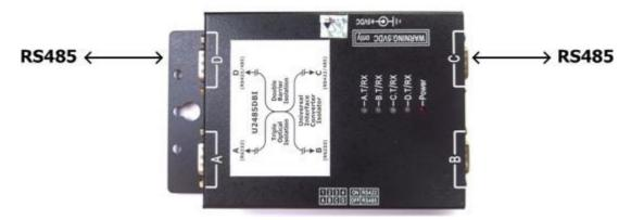
We can use port D as RS485 input (DIP Switch bit4 set in OFF location) and port C as RS485 output (DIP Switch bit3 set in OFF location) to split RS485 network for more nodes support and connection range.
