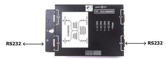
We can use port A as RS232 input and port B as RS232 output (DIP Switch bit2 set in OFF location) to let two RS232 devices with Ground isolated connection.
