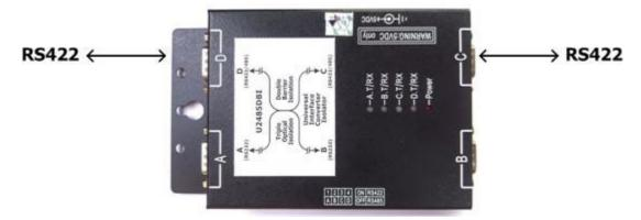
We can use port D as RS422 input (DIP Switch bit4 set in ON location) and port C as RS422 output (DIP Switch bit3 set in ON location) to extend the connection range.
