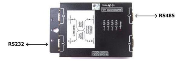
We can use port A as RS232 input and port C as RS485 output (DIP Switch bit3 set in OFF location) to let one RS232 device to work in RS485 network environment.
