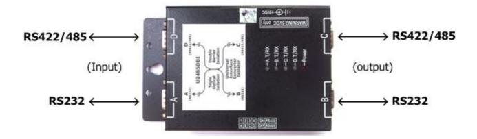
When one user needs to have long distance communication capability, we can use full-duplex RS422 interface or half-duplex RS485 interface. In U2485DB-I box we can set each serial port to target RS422 interface mode or RS485 interface mode vi DIP SWITCH anytime.
