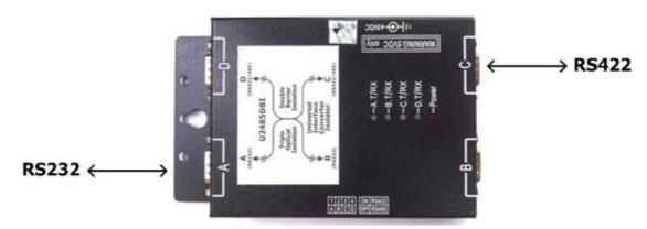
We can use port A as RS232 input and port C as RS422 output (DIP Switch bit3 set in ON location) to have long distance full-duplex communication capability.
