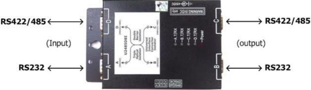
1. We can have DIP Switch to set each serial port interface type. Bit 1 is used for port A, Bit 2 is used for port B, Bit 3 is used for port C, Bit 4 is used for port D. When we set in ON location, it is in RS422 interface mode. When we set in OFF location, it is in RS485 interface mode.
