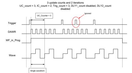
Figure 4-16: Post-Trigger or Delayed-Trigger with Retriggering
