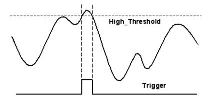
Figure 4-5: Above-High Analog Triggering
