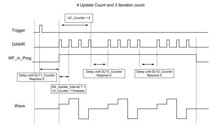
Figure 4-13: Waveform Generation Hardware Timing
