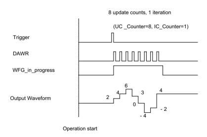
Figure 4-14: Post-Trigger Waveform Generation
