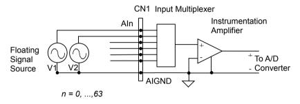
Figure 2-15: Floating source w/ RSE input connections
