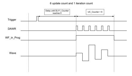
Figure 4-15: Delayed-Trigger Waveform Generation
