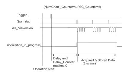
Figure 4-8: Delayed Trigger
