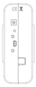
Figure 2-1: USB-1902 Module Rear View
