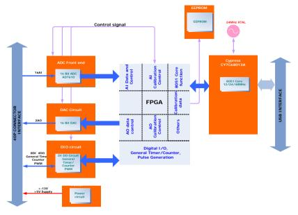
Figure 4-1: Functional Block Diagram (USB-1902)
