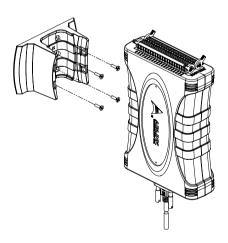
Figure 2-14: Module with Wall Mount Apparatus
