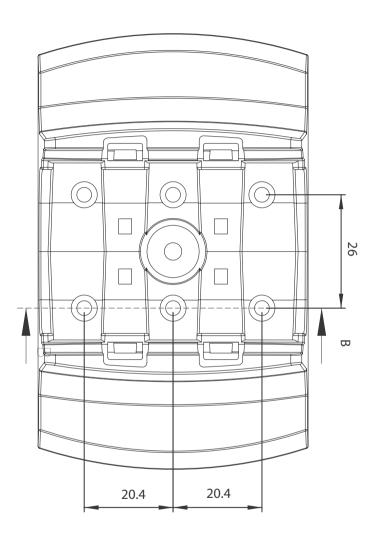
Figure 2-7: Module Stand Top View
