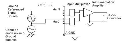
Figure 2-16: GRND-Referenced Sources w/ NRSE Inputs
