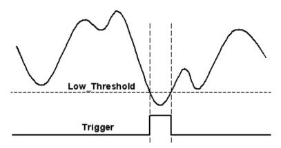
Figure 4-4: Below-Low Analog Triggering
