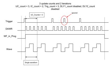
Figure 4-9: Post Trigger or Delay Trigger with Retriggering
