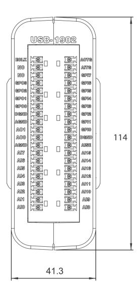
Figure 2-3: USB-1902 Module Front View
