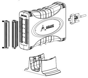
Figure 2-4: Module, Stand, Connector, and USB Cable
