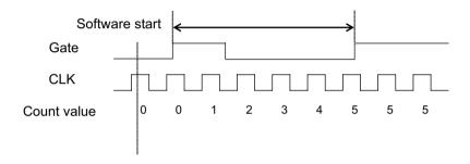
Figure 4-19: Mode 2-Single Period Measurement
