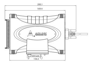
Figure 2-5: Module, Stand, & Wall Mount Kit Side View (w/ connections)
