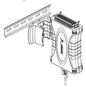
Figure 2-11: Module Pre-Rail Mounting
