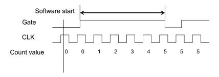
Figure 4-20: Mode 3-Single Pulse-Width Measurement
