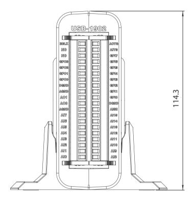
Figure 2-6: Module in Stand Front View
