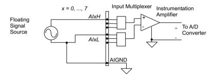
Figure 2-18: Floating Source w/ P-D Input
