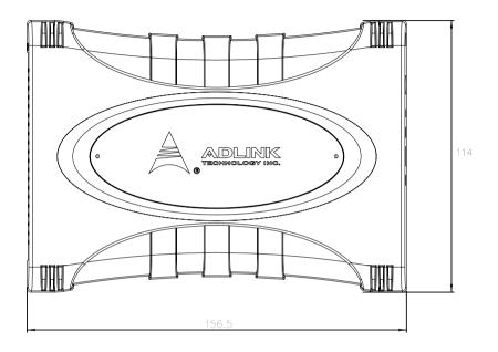
Figure 2-2: USB-1902 Module Side View
