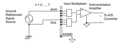
Figure 2-17: GRND-Referenced Source w/ P-D Input
