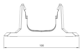
Figure 2-9: Module Stand Front View
