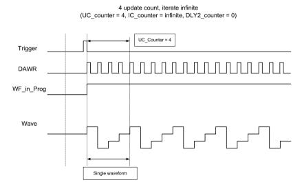
Figure 4-17: Infinite Iteration Waveform Generation
