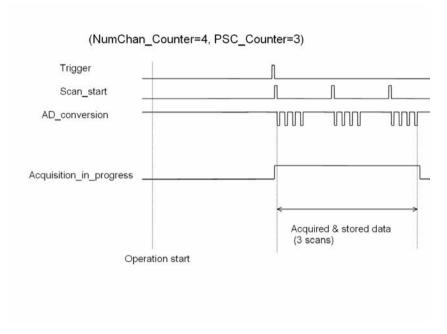
Figure 4-7: Post Trigger without Retriggering
