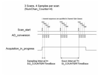
Figure 4-3: Analog Input Scan Timing
