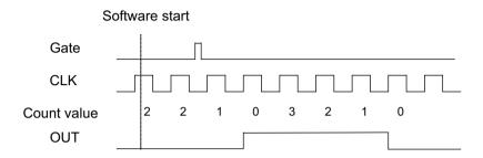
Figure 4-22: Mode 5-Single-Triggered Pulse
