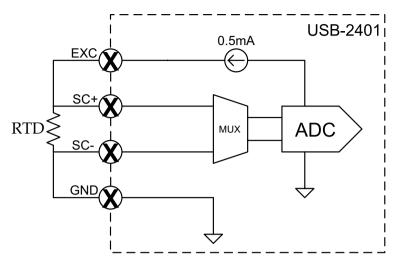
Figure 3-7: 4-Wire RTD Connection
