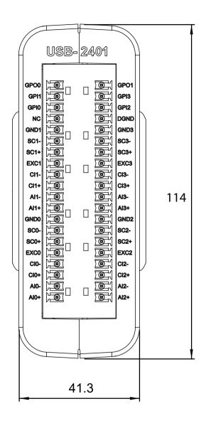
Figure 1-4: USB-2401 Module Front View
