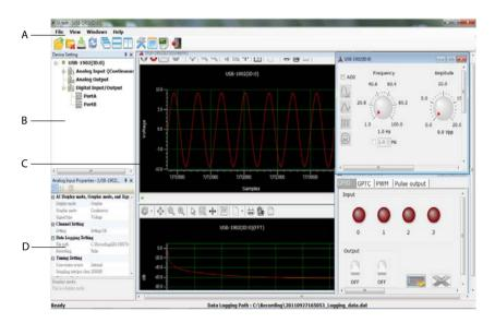
Figure 1-1: U-Test Interface
