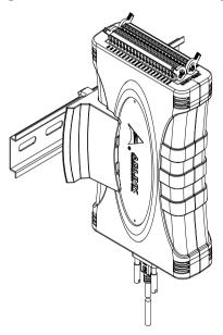
Figure 2-5: Module Rail-Mounted
