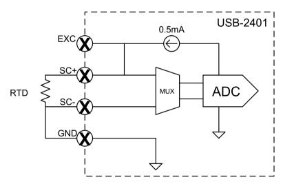
Figure 3-8: 3-Wire RTD Connection
