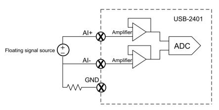
Figure 3-3: Floating Source and Differential Input
