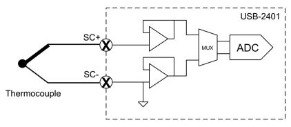
Figure 3-6: Thermocouple Connection
