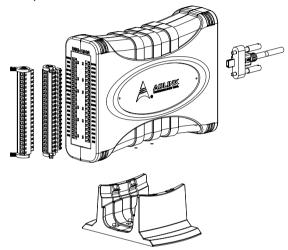
Figure 1-5: Module, Stand, Connector, and USB Cable
