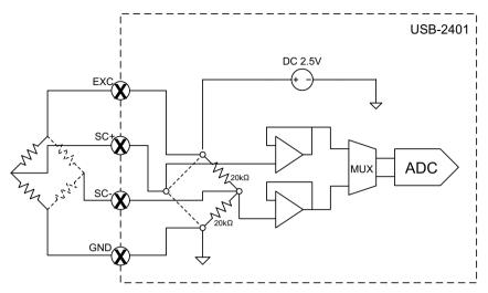
Figure 3-5: Full Bridge and Half Bridge Connection
