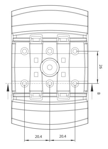
Figure 1-8: Module Stand Top View
