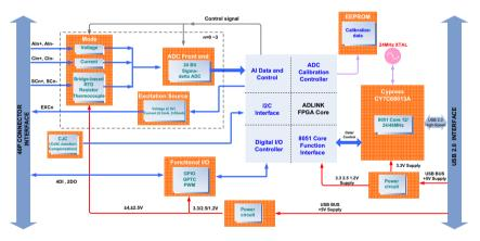
Figure 3-1: USB-2401 Functional Block Diagram
