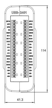
Figure 1-2: USB-2401 Module Rear View
