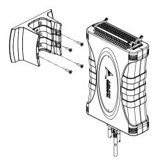
Figure 2-7: Module with Wall Mount Apparatus
