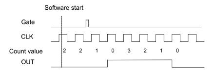
Figure 3-15: Mode 5-Single-Triggered Pulse
