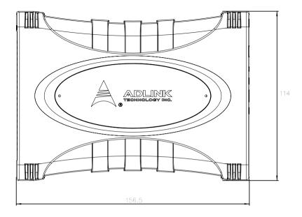
Figure 1-3: USB-2401 Module Side View
