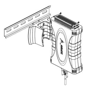
Figure 2-4: Module Pre-Rail Mounting
