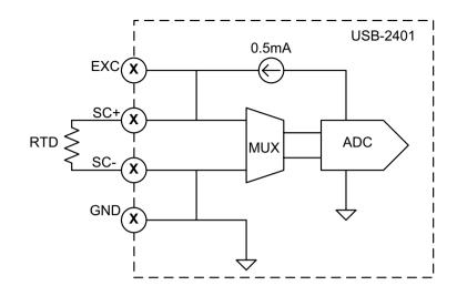
Figure 3-9: 2-wire RTD Connection
