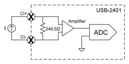
Figure 3-4: Current Source Connection
