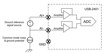
Figure 3-2: Ground-Referenced Source and Differential Input
