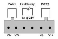
Step 1: insert the negative/positive wires into the V-/V+ terminals, respectively.
