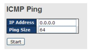
After you press **Start**, five ICMP packets will be transmitted, and the sequence number and roundtrip time will be displayed upon reception of a reply. The page refreshes automatically until responses to all packets are received, or until a timeout occurs.
