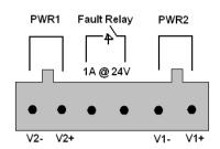
Step 2: to keep the DC wires from pulling loose, use a small flat-blade screwdriver to tighten the wire-clamp screws on the front of the terminal block connector.
