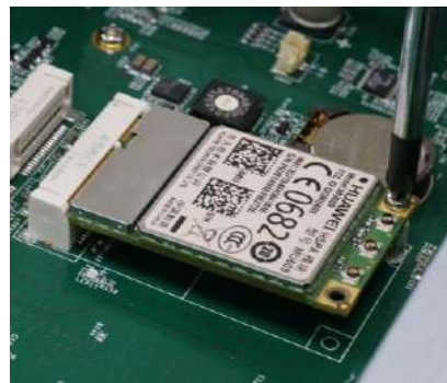
Secure the module with a screw
