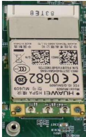
Insert on 45 degree angle
